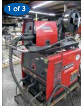
(3) LINCOLN CV-305 ELECTRIC WELDER
