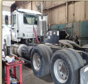
2013 MACK CHU613 T/A TRUCK TRACTOR W/ MACK MP8 505HP, 18 SP FULLER, 14,000 LB FRONT AXLE, 40,000 LB REARS, AIR RIDE SUSP, MILES READ VIN 1M1AN07YXDM013399
