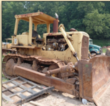
1975 CAT D8H CRAWLER DOZER W/ ROPS CANOPY, 4-WAY BLADE, POWER SHIFT, HRS READ, S/N 46A33000
