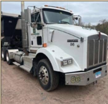
2014 KW T800 T/A TRUCK TRACTOR W/ PACCAR ENG, 12,000 LB FRONT AXLE, 40,000 LB REAR AXLE, VIN 1XKDDP9X6EJ404053
