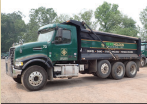
(2 OF 3) 2017 VOLVO VHD TRI/A DUMPS, VOLVO D13 455 HP ENG, AUTO I-SHIFT, 20K FA, 20K STEERABLE LIFT, 46K REARS, 17 1/2 FT STEEL DUMP, MILES READ 328,435, VIN 4V5K99EH8HN984787
