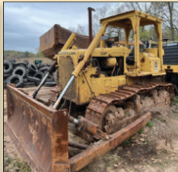
1985 CAT D6D CRAWLER DOZER; ROPS CANOPY, 4-WAY BLADE, S/N 4X10094
