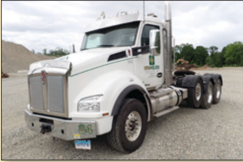
2021 KW T880 TRI/A TRUCK TRACTOR, CUMMINS X-15 600 HP, 18 SP TRANS, 20,000 LB FRONT AXLE, 20,000 LB STEERABLE AIR LIFT AXLE, 46,000 LB REAR AXLE, AUX HYD, AIR RIDE SUSP, ALUM HEADACHE RACK, STROBE LIGHTS, POLISHED ALUM WHEELS, AIR TO THE REAR, 86,000 GVWR, MILES READ 117,430, VIN 1XKZP4TX4MJ445266
