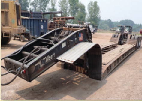
2007 TALBERT LOWBED; 55 TON, TRI/A, LEVEL DECK, 26 FT WELL, VIN 40FSK574471027213
