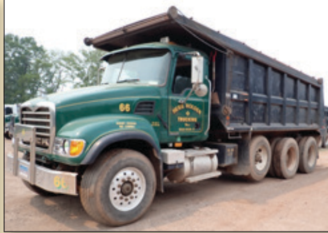
(1 OF 4) 2006 -2004 MACK CV-713 GRANITE TRI/A DUMPS; MACK E7 400 HP, 10 SP, 20,000 LB FRONT AXLE, 20,000 LB NON-STEERABLE LIFT AXLE, 46,000 REAR AXLE, 17 1/2 FT BODY, MILES READ 649,683, VIN 1M2AG11C44M009213
