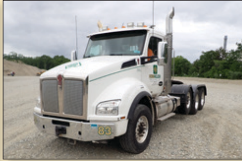
2019 KW T880 TRI/A TRUCK TRACTOR, CUMMINS X-15 600 HP, 18 SP TRANS, 20,000 LB FRONT AXLE, 20,000 LB STEERABLE AIR LIFT AXLE, 52,000 LB REAR AXLE, AUX HYD, AIR RIDE SUSP, ALUM HEADACHE RACK, STROBE LIGHTS, POLISHED ALUM WHEELS, AIR TO THE REAR, 92,000 GVWR, MILES READ 163,784, VIN 1XKZP4TX7KJ283761
