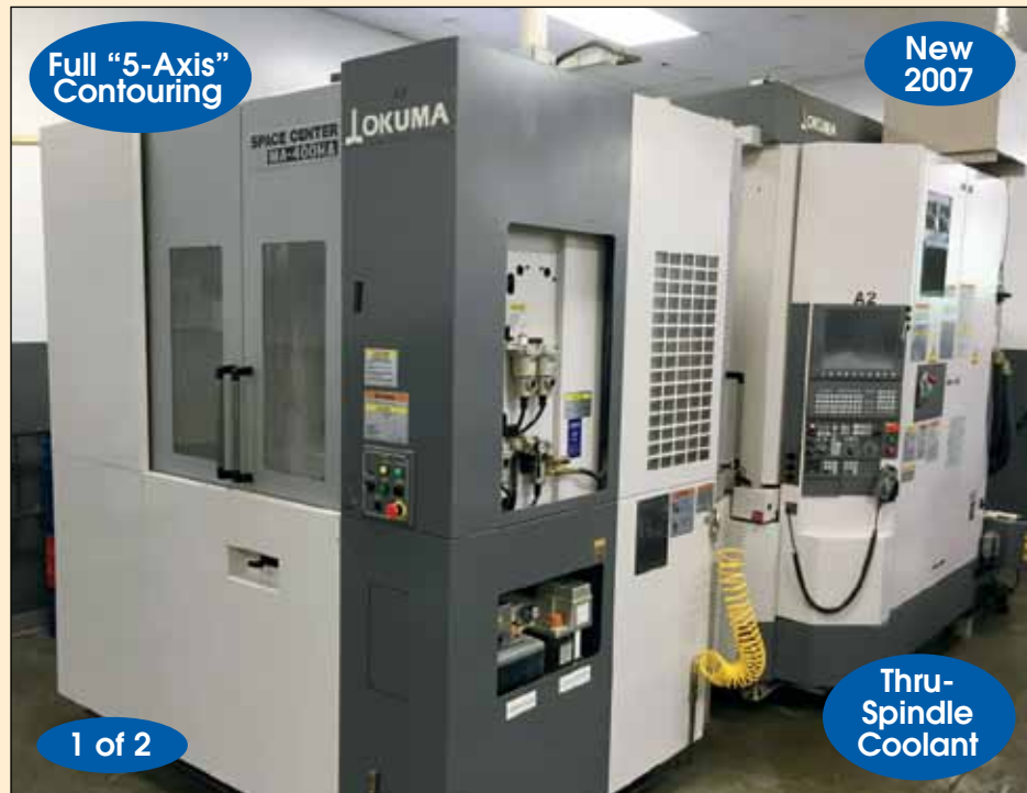
OKUMA # MA-400HA "5-AXIS" CNC HORIZONTAL MACHINING CENTER W/ TSUDAKOMA 5TH-AXIS ROTARY TABLES
