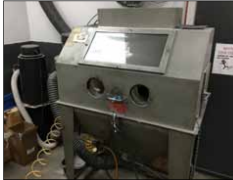
SAND BLAST W/ DUST COLLECTOR
