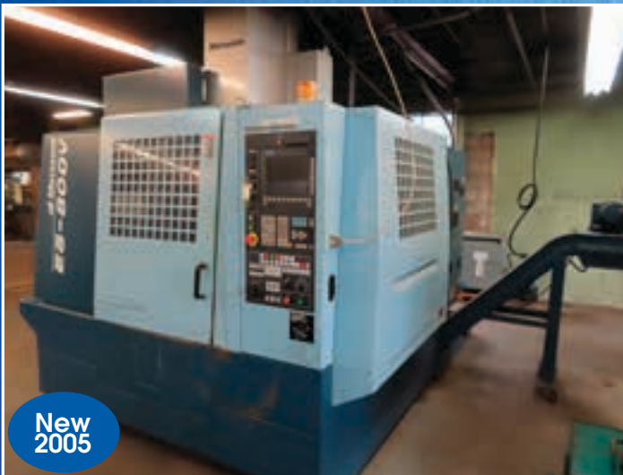
Matsuura 3 Axis Vertical Machining Center Model ES800V
