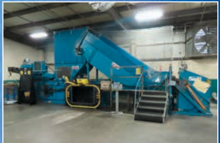
Summit Baler Model PR-9S, Hydraulic Auto Dumper & Conveyor, 70 HP
