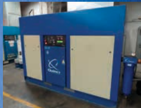
QUINCY 125 HP ROTARY SCREW AIR COMPRESSOR MODEL QSI-600
