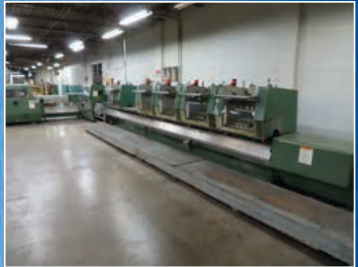
Muller Martini Prima Saddle Stitcher 6-Pk, Cover Feeder, 3-Knife Trimmer
