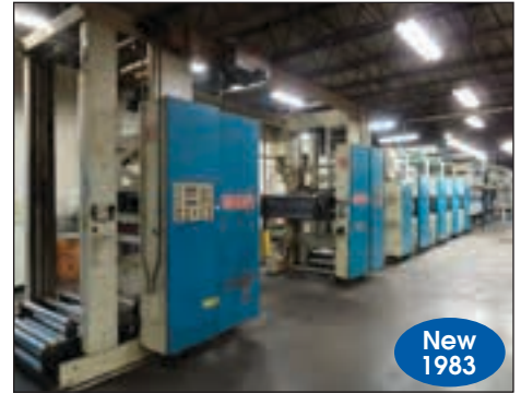
HARRIS M-300 WEB PRESS, 22 3/4" CUTOFF, 36" WEB WIDTH
