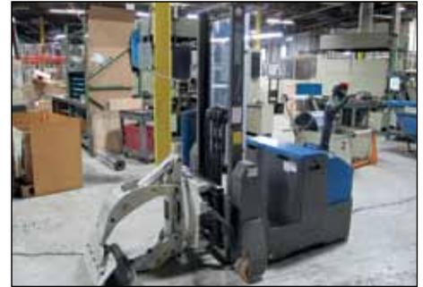
Armani Model DCP100/Walk Behind Pallet lift //Cascade Barrel Clamp, 2425 Lb,@21"
