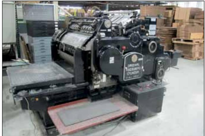
Original Heidelberg Cylinder Die Cutter Model SBB 22.5" X 32.25"
