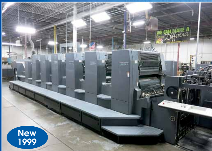
Heidelberg 6-Color Sheet Fed Printing Press Model CD102-6+L
