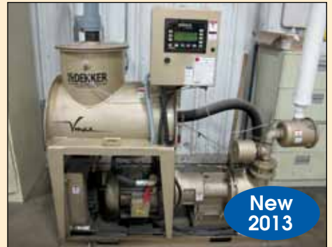
DECKER VACUUM PUMP
